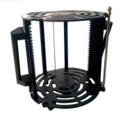
**Recif Technologies** MCs offers ergonomic solution for thermal processes applications. Made of a special aluminium alloy, it gurantees high mechanical performances
